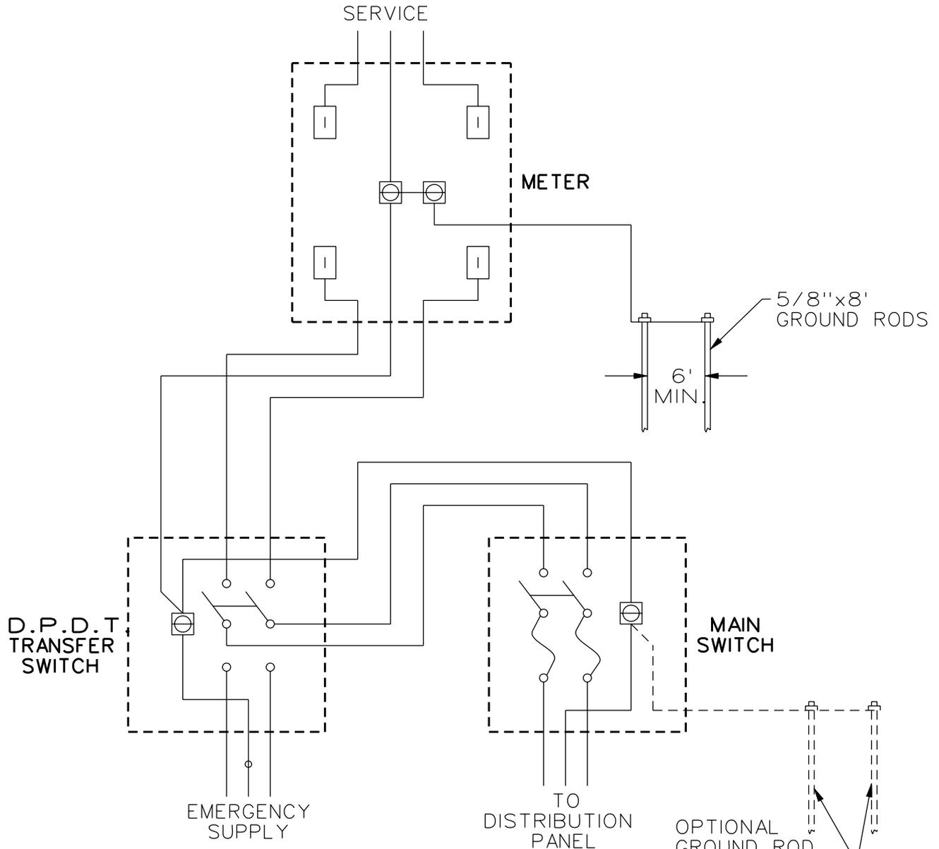
DOUBLE POLE DOUBLE THROW (D.P.D.T.) TRANSFER SWITCH INSTALLED BETWEEN METER AND MAIN SWITCH. TRANSFER SWITCH MAY BE MANUAL OR AUTOMATIC.
