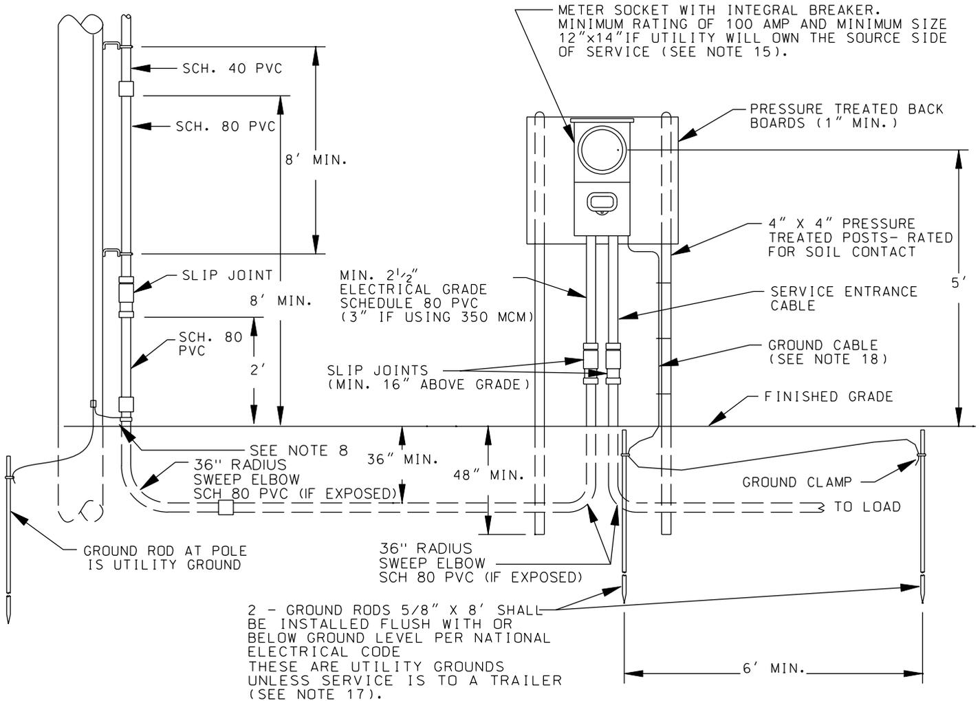
2 - GROUND RODS 5/8" X 8' SHALL BE INSTALLED FLUSH WITH OR BELOW GROUND LEVEL PER NATIONAL ELECTRICAL CODE THESE ARE UTILITY GROUNDS UNLESS SERVICE IS TO A TRAILER (SEE NOTE 17).
