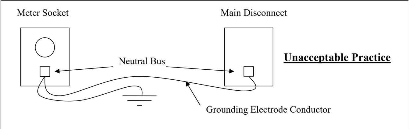
B. Typically the meter socket's neutral buss is bonded to the meter socket's steel case. That bond shall satisfy the requirement to connect the meter sockets steel case to ground. If the neutral buss is not connected to the meter socket's steel case, then install a bonding jumper to connect the case. (*Exception- Check with your local Utility to confirm whether a bonding jumper to the pole downground, on a pole meter, is required or disallowed.*)
